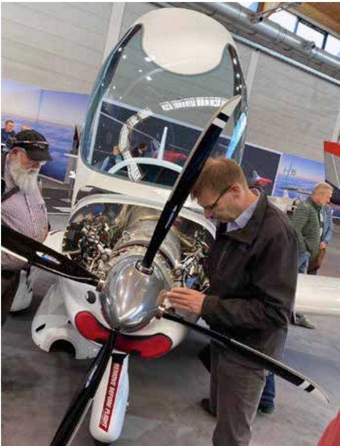
Small 140 HP Turbine on a Bristell aircraft
